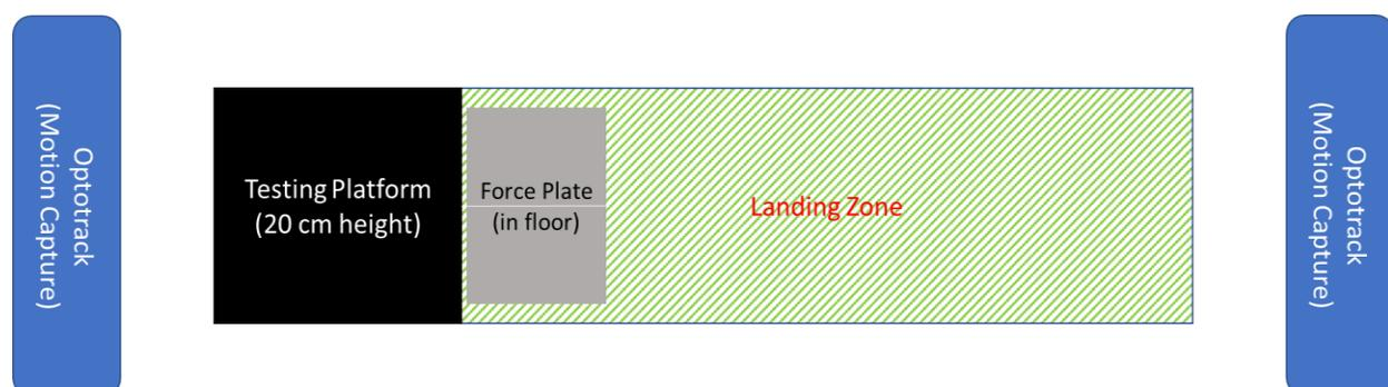
Figure 1: Lab setup to capture ground reaction force and horizontal displacement during the U-HDJ assessment.
